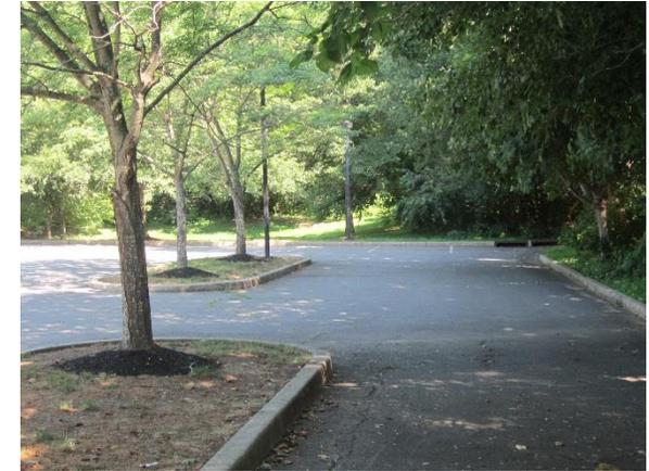
Parking spots west of the office suites can be replaced with porous asphalt to capture and infiltrate stormwater. A preliminary soil assessment suggests that the soils have suitable drainage characteristics for green infrastructure.
