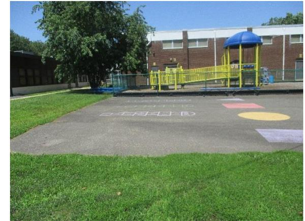
Multiple areas of pavement surrounding the school can be replaced with porous asphalt to capture and infiltrate stormwater. A rain garden can be installed adjacent to the paved playground to capture, infiltrate and treat runoff. A preliminary soil assessment suggests that the soils have suitable drainage characteristics for green infrastructure.
