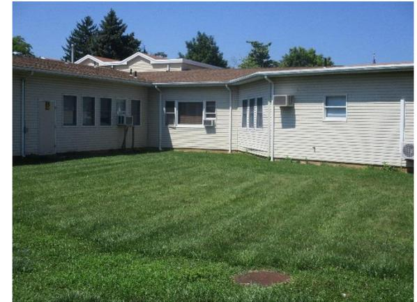
Parking spots south of the church can be replaced with porous asphalt to capture and infiltrate stormwater. Bioretention systems can be installed north of the church to capture, treat, and infiltrate rooftop runoff. A preliminary soil assessment suggests that the soils have suitable drainage characteristics for green infrastructure.
