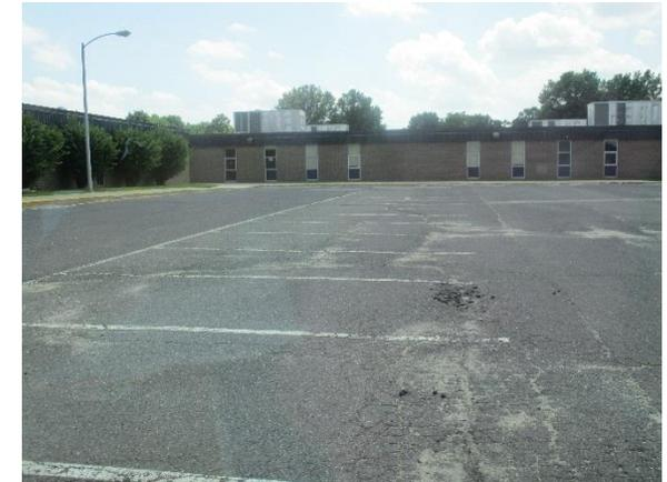
Stormwater is currently directed to an existing detention basin. Parking spots can be replaced with porous asphalt to capture and infiltrate stormwater. A preliminary soil assessment suggests that more soil testing would be required before determining the soil's suitability for green infrastructure.
