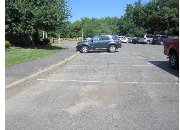
Stormwater is currently directed to an existing detention basin. Parking spots near the basketball courts can be replaced with porous asphalt to capture and infiltrate stormwater. A rain garden can be installed adjacent to the pavilion to capture, treat, and infiltrate roof runoff. A preliminary soil assessment suggests that the soils have suitable drainage characteristics for green infrastructure.
