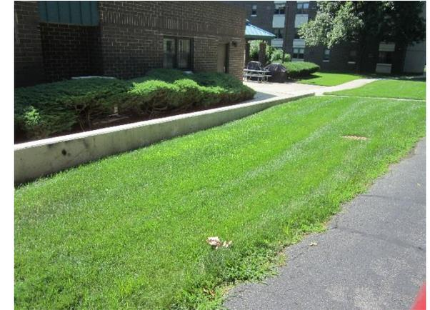
Parking spots north of the building can be replaced with porous asphalt to capture and infiltrate stormwater. A rain garden adjacent to the west side of the building can capture, treat, and infiltrate runoff. A preliminary soil assessment suggests that the soils have suitable drainage characteristics for green infrastructure.
