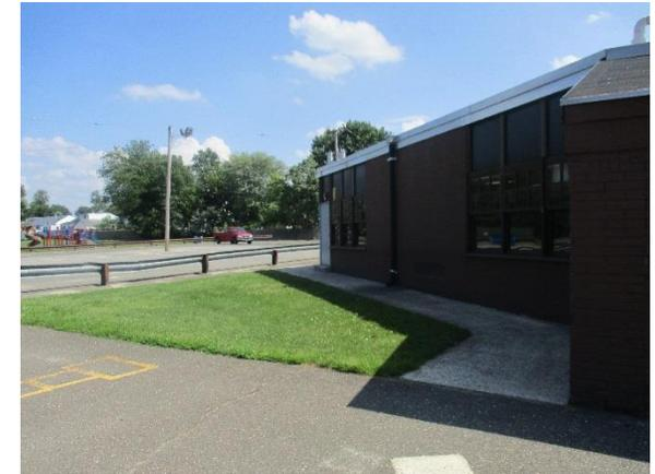
Stormwater is currently directed to an existing detention basin. Parking spaces by the northern building can be replaced with porous asphalt to capture and infiltrate stormwater. A bioretention system can be installed adjacent to the driveway to capture, treat, and infiltrate rooftop runoff. A preliminary soil assessment suggests that more soil testing would be required before determining the soil's suitability for green infrastructure.
