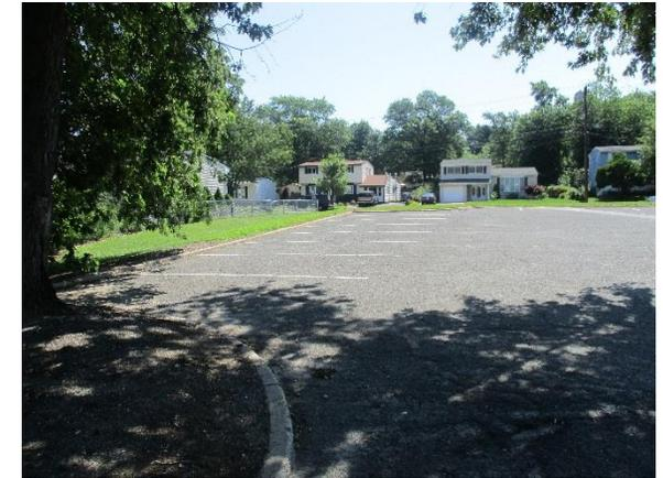
Parking spots northeast of the school can be replaced with porous asphalt to capture and infiltrate stormwater. A rain garden can be installed to capture, treat, and infiltrate rooftop runoff. A preliminary soil assessment suggests that the soils have suitable drainage characteristics for green infrastructure.
