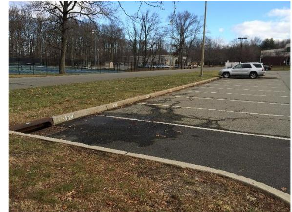
Multiple rows of parking spaces around the complex can be replaced with porous asphalt to capture and infiltrate stormwater. A rain gardens can be installed east of the library to capture, treat, and infiltrate roof runoff. A preliminary soil assessment suggests that more soil testing would be required before determining the soil's suitability for green infrastructure.
